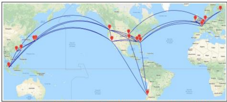
Figure 1: B4 global topology. Each marker indicates a site or multiple sites located in close geographical proximity. B4 consists of 33 sites as of January, 2018.
